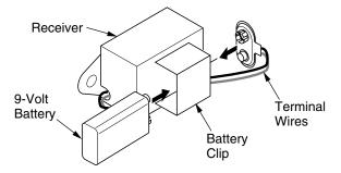
Figure 48 - Installing Battery in Receiver
